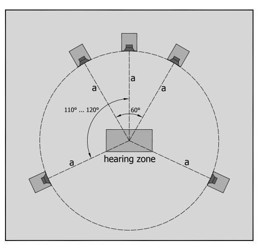
• Distance between speakers and your listening position  $a = 2m \dots 4m (6'7'' \dots 13'1'')$ In case installation in the prescribed way is not possible in your listening room most decoding devices allow adjustments of single speakers.
